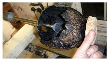
First, loosen the taper plug and slide to the head stock end. Place your hollow form onto the jig. Bring up the tail stock and centre into the waste wood. Lock tail stock and tighten against the inside blue foam. This puts all of the pressure at the bottom of the hollow form preventing spiting of the neck.
