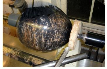
The bottom of the hollow form can now be turned down to a finish. A small central "dimple" should be left about 15mm minimum (depending of wood type). This can be cut away and sanded to a finish, off the lathe. Max recommended RPM ,1500.
