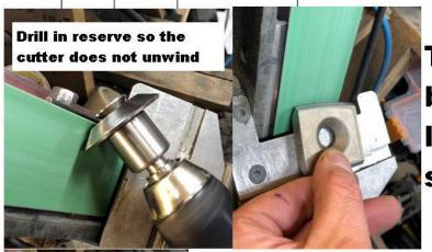
To sharpen from blunt, first grind the long bevel, then short bevel.
